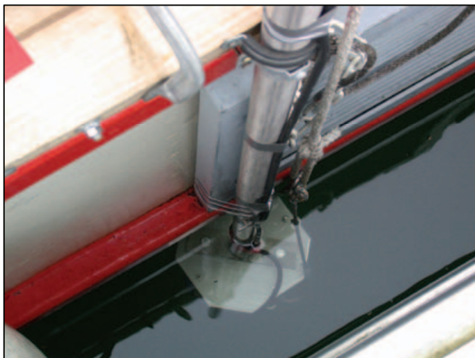
Fig.2 Acoustic Doppler Current Profiler (ADCP) mounted aside the RV „Komoran“.
